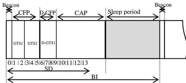
Figure 3 : Superframe structure according to FF-MAC protocol
