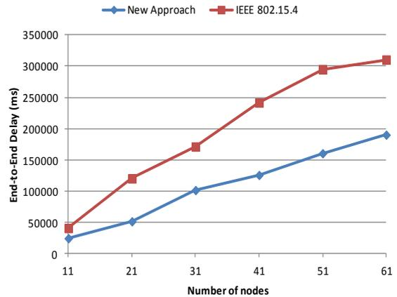
Figure 9: End-to-End delay for different network sizes
