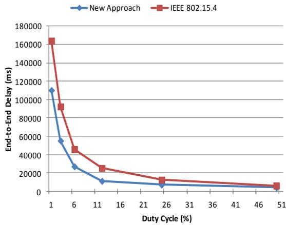
Figure 8: End-to-End delay vs. duty cycle (51 nodes)
