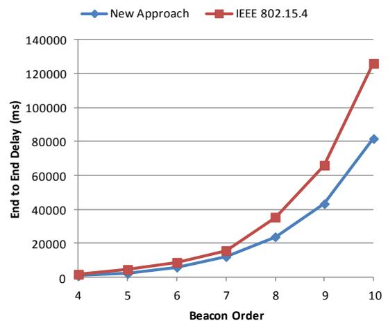
**Figure 7: End-to-End delay vs. beacon order (31 nodes, SO=4)**
