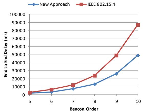
**Figure 6: End-to-End delay vs. beacon order (21 nodes, SO=5)**
