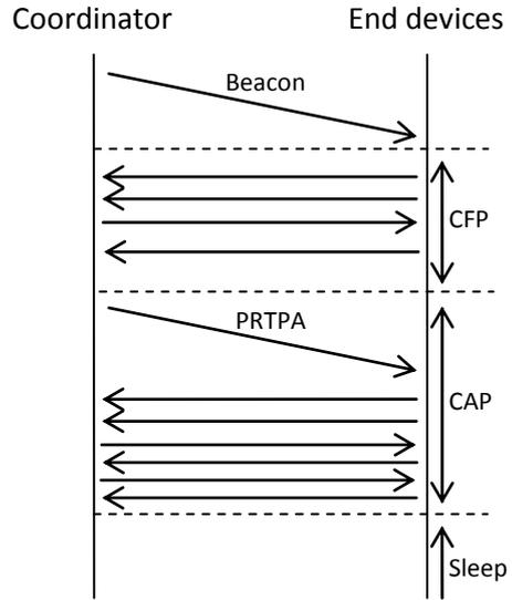
Figure 4 : Message sequence chart describing the packet exchange timing
